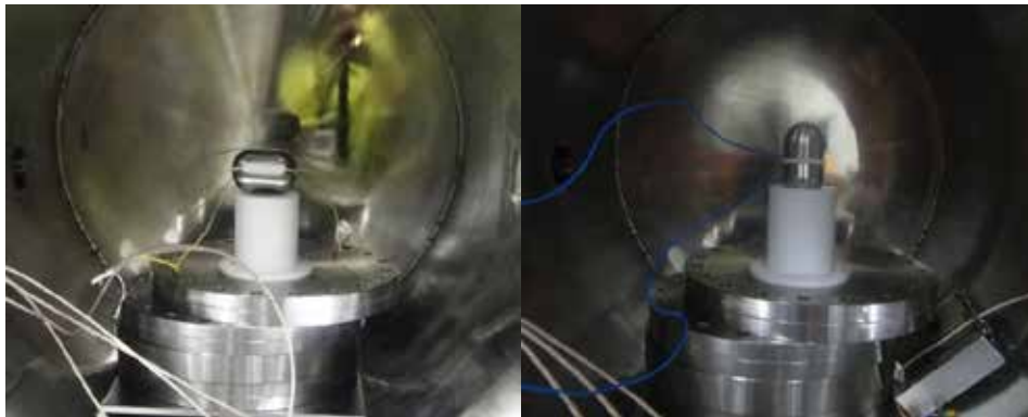
Figure 27: LP prototypes mounted in the vacuum chamber horizontally (left) and vertically (right).
