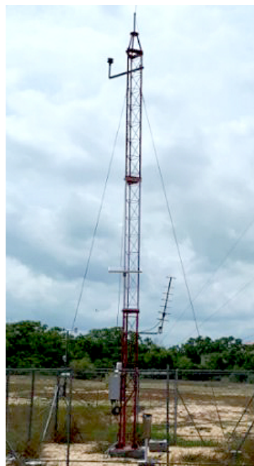
Figure 9: ISRO's Automatic Weather Station installed at TERLS
