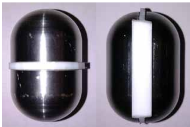
Figure 26: LP prototypes of same dimensions (50 mm long \times 30 mm wide) partitioned horizontally and vertically. The two partitions are mechanically integrated but electrically insulated (white colour, Teflon) with each other.
