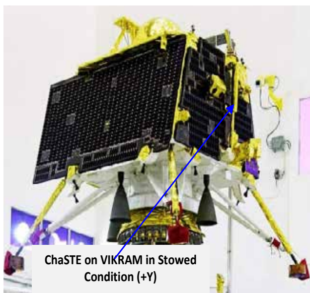
Figure 10: ChaSTE payload in stowed condition on the + Y panel of lander VIKRAM
