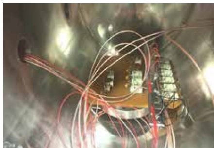
Figure 2: CEM detectors kept inside vacuum chamber for burn-in test.
