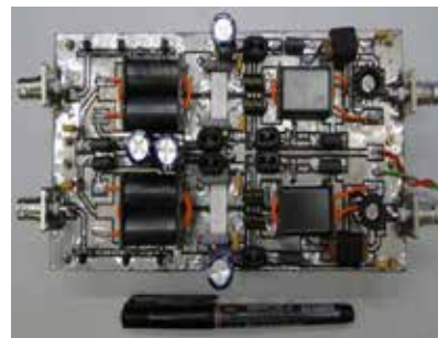
Figure 3: 300 W RF power amplifier developed for Digisonde.
