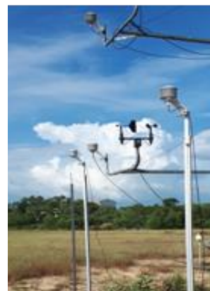
Figure 9: Set-up for comparing the meteorological sensors.
