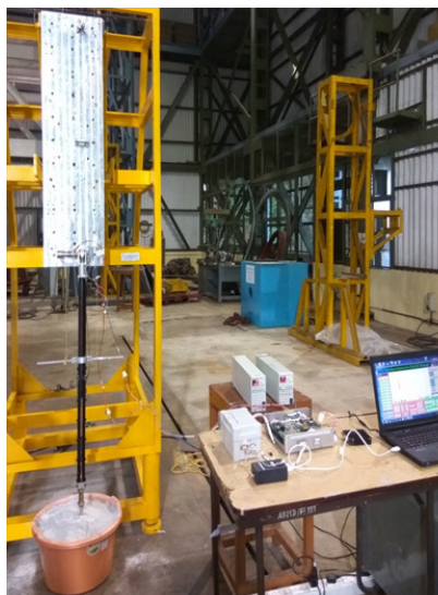
Figure 11: Engineering model of ChaSTE Payload undergoing functional tests.
